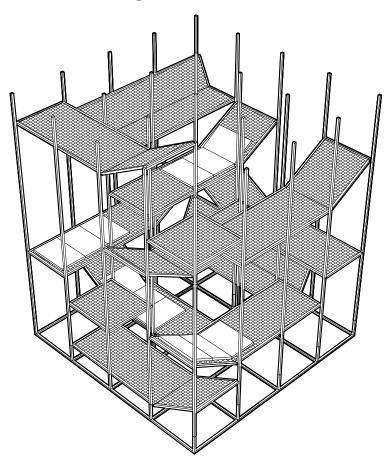
Powder coated metal frame in Fluo Yellow (RAL 1016) Mesh Galvanized
